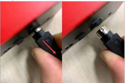
For the rectangular adapter, press the button on top of the connector to release the connector and pull from the base of the connector. Pulling from the cord could damage the adapter.
